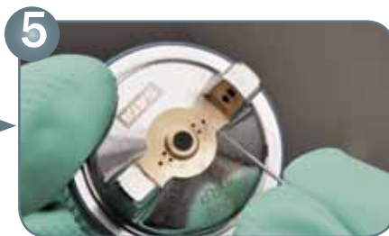
5 Ideally, please use specially designed SATA cleaning brushes and SATA nozzle cleaning needles to ensure optimum
