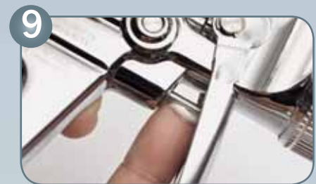
Grease visible part of air piston rod
