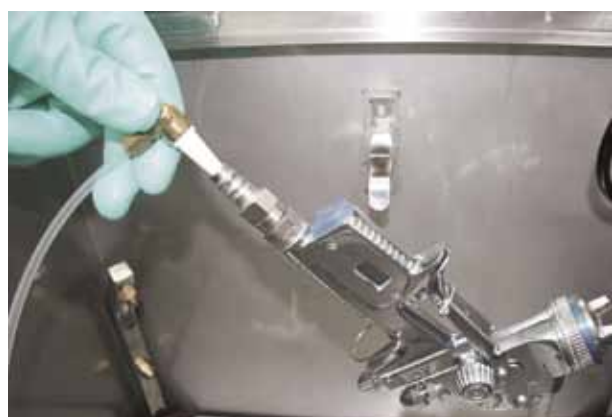
2. Connect air connection to air inlet
