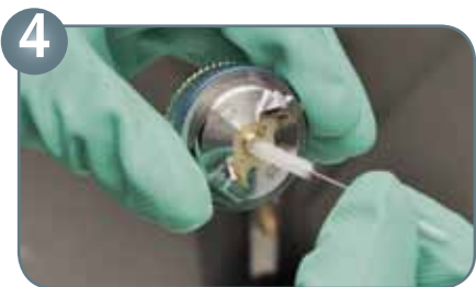
4 When cleaning the nozzle components, please make sure that metal parts of brushes do not damage the nozzle set.
