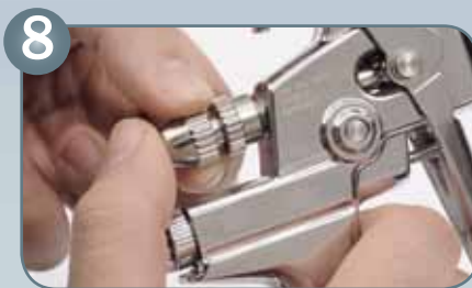
Install material flow control screw
