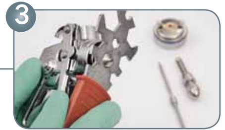
3 And finally, unscrew fluid tip with the ring spanner integrated in the universal spanner.
