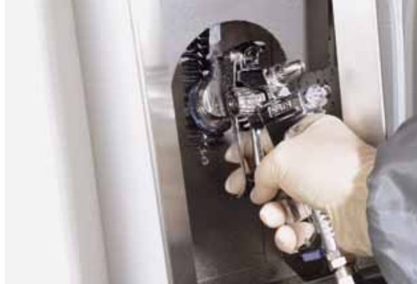
1. Cleaning of material passage and air cap
